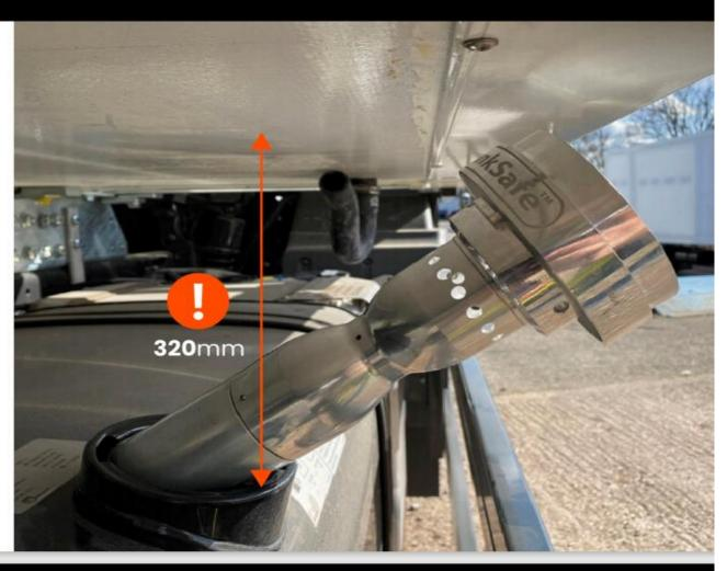
Minimum clearance required for filling the TankSafe® Optimum device when fitted to a rigid vehicle
